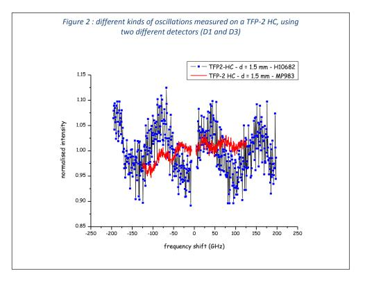
These observations all play in favour of the idea that this effect is introduced by the detector. If this was the correct explanation, the oscillation would be maximum if the light falling on the detector were parallel.
